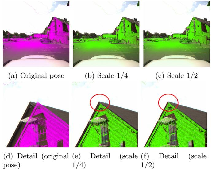
Figure 10: Coarse Registration comparison on Council street data, with initial registration error of  $2.4^\circ$  (yaw) and  $0.5^\circ$  (pitch). Magenta color is the original registration and green color is the coarse registration results at different scale. The computation took around 60s.
