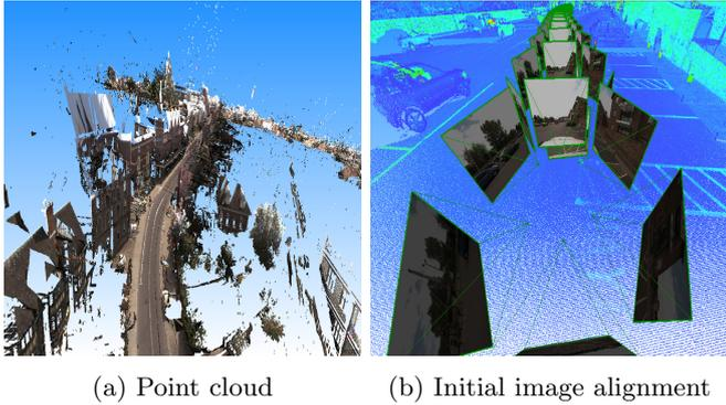
Figure 1: Example data, taken using a mobile LiDAR with mounted camera in the town of Shrewsbury (UK)
