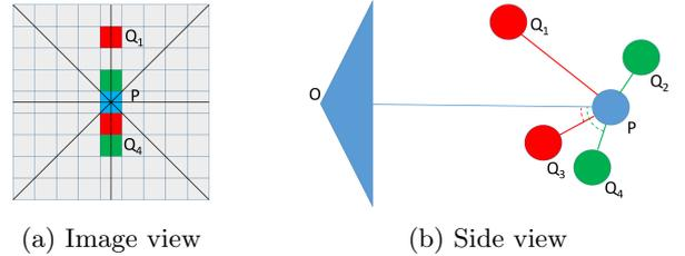
Figure 4: Projection of 5 points onto an image. The considered point and its projection on a pixel are depicted in blue. The visibility angle is the angle  $\langle \vec{OP}, \vec{QP} \rangle$ . An horizon pixel is a pixel corresponding to the point with the smallest angle in a sector. These pixels are depicted in red, they are the points that best occlude the central point. Other pixels are in green.
