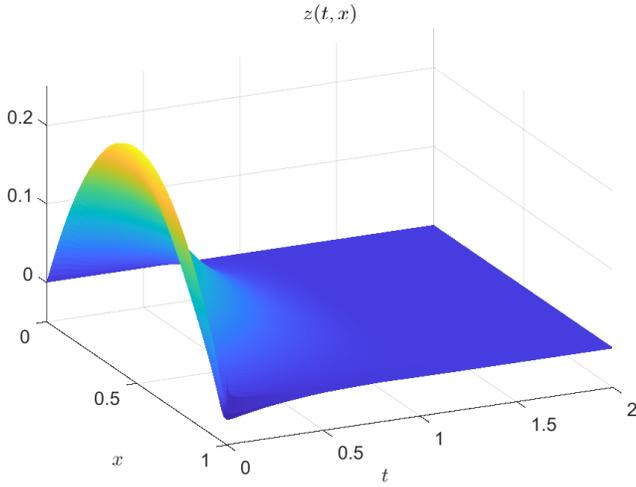
Fig. 4. The evolution of the state  $z(t, x)$  of the closed-loop system (6) with the control  $U(t)$  in (11) with  $\mathcal{K}(V(z(t, \cdot))) = c_1 V(z(t, \cdot))^\alpha + c_2 V(z(t, \cdot))^\beta$ , for the initial condition  $z(t_0, x) = x - x^2$ ,
