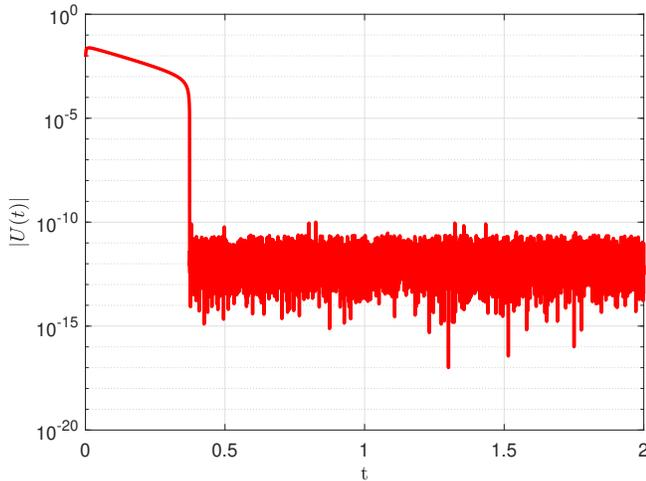
Fig. 2. The evolution of the nonlinear control  $U(t)$  given in (11) with  $\mathcal{K}(V(z(t, \cdot))) = cV(z(t, \cdot))^\alpha$  for the initial condition  $z(t_0, x) = x - x^2$ .
