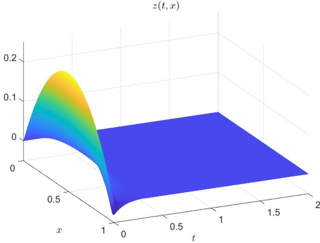
Fig. 1. The evolution of the state  $z(t, x)$  of the closed-loop system (6) with the control  $U(t)$  in (11) with  $\mathcal{K}(V(z(t, \cdot))) = cV(z(t, \cdot))^\alpha$ , for the initial condition  $z(t_0, x) = x - x^2$ ,
