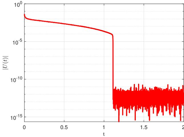
Fig. 5. The evolution of the nonlinear control  $U(t)$  given in (11) with  $\mathcal{K}(V(z(t, \cdot))) = c_1 V(z(t, \cdot))^\alpha + c_2 V(z(t, \cdot))^\beta$  for the initial condition  $z(t_0, x) = x - x^2$ .
