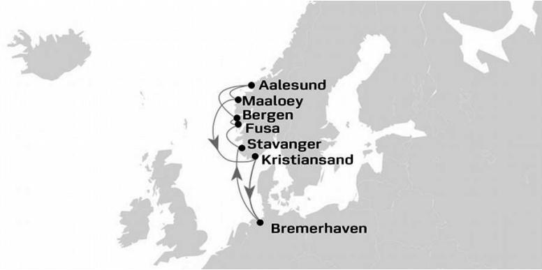
Figure 4.2: A feeder service collect containers in the hub in Bremerhaven and transport them to their destinations in Norway.
