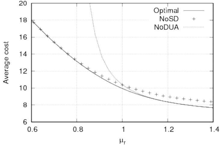
Figure 13: Effect of remanufacturing rate  $\mu_r$  on the average cost when  $\{\lambda = 1, \delta = 0.8, h = 1, h_r = 0.95, b = 3, \mu = 10, c_m = 10, c'_a = 1, c_r = 1, c_e = 30, c_d = 1, \alpha = 0\}$ .
