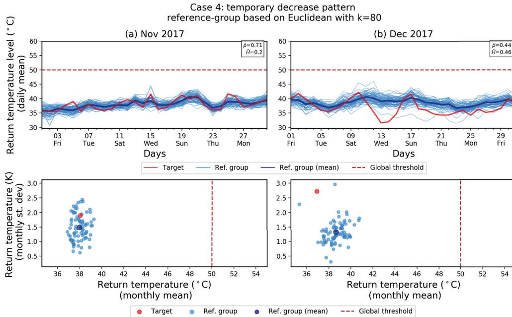
**Figure 9:** Example case of the "temporary decrease" pattern: A decrease in the return temperature of the target was observed for a few weeks of Dec'17 in comparison to its reference-group.
