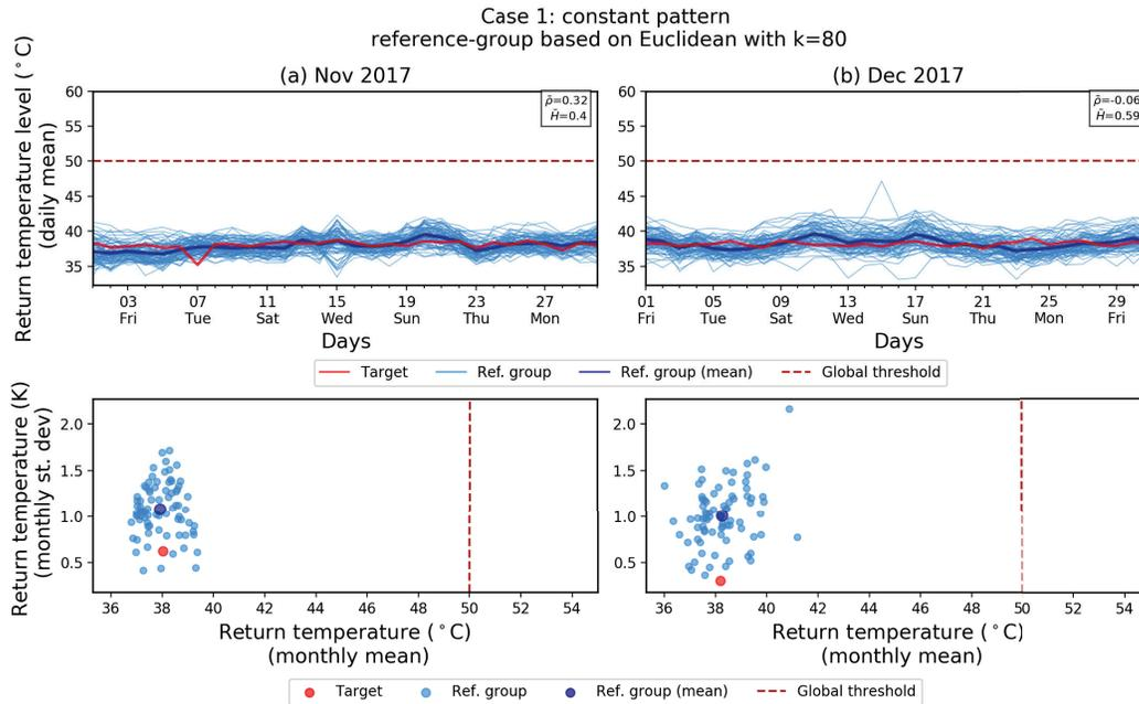
**Figure 6:** Example case of the "constant" pattern: The return temperature of the target stays at near constant levels compared to its reference-group.
