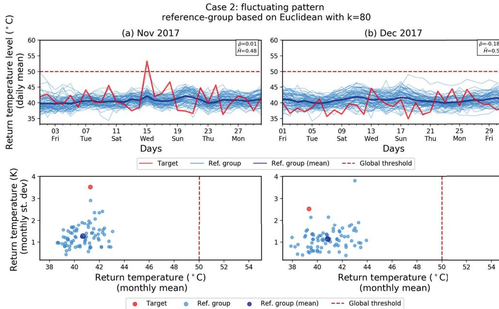
**Figure 7:** Example case of the "fluctuating" pattern: A possible malfunctioning target substation, which shows erratic behavior with high variability compared to its reference-group.
