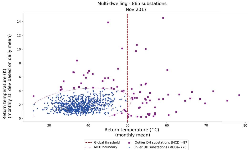
**Figure 1:** Based on the global threshold, 52 (5.9% contamination rate) substations had a monthly mean return temperature greater than 50°C in Nov'17. MCD discovered 87 outlier substations based on a contamination rate of 0.1 or 10%.
