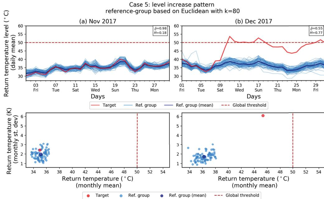
**Figure 10:** Example case of the "level increase" pattern: An abrupt increase in the return temperature of the target was observed in comparison to the reference-group in Dec'17. This could possibly be due to a fault in the flow control valve.
