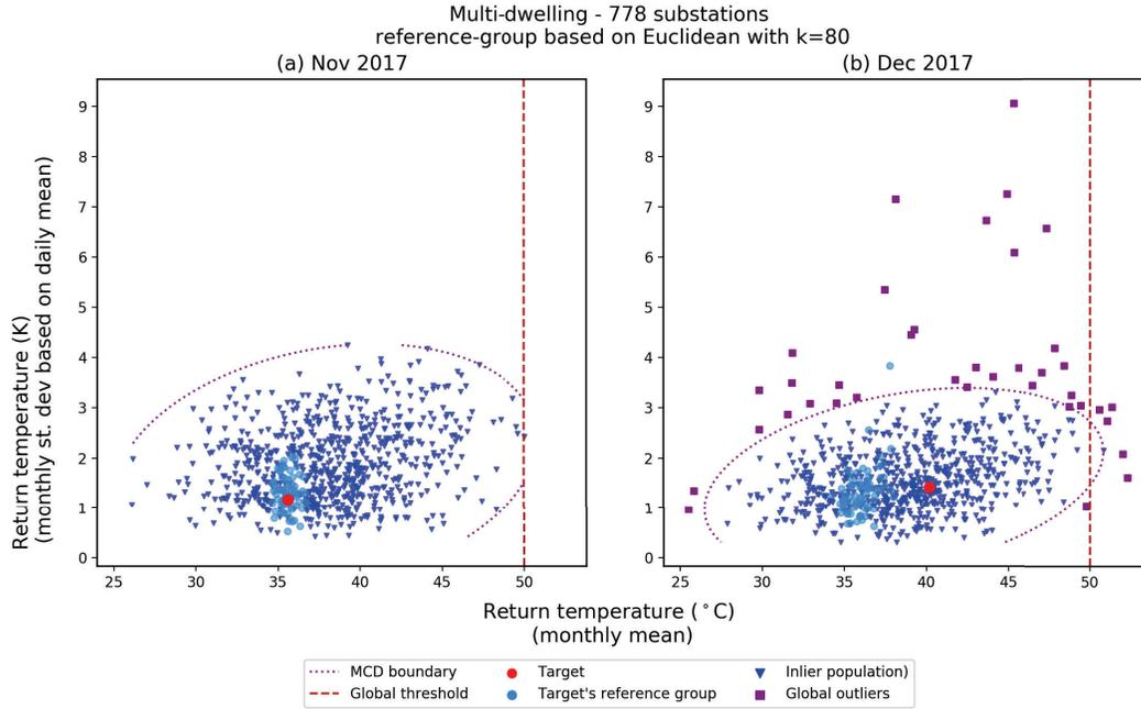
**Figure 5:** (a): The target substation (red dot) in Nov'17, relative to its reference (light blue dots) and population (blue dots) is shown. (b): The target substation relative its reference-group and population in Dec'17 is shown.
