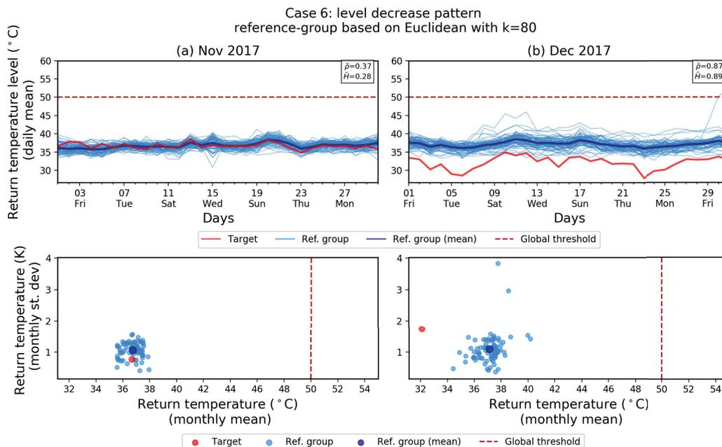
**Figure 11:** Example case of the "level decrease" pattern: A considerable decrease in observed in the return temperature of the target compared to its reference-group. This indicated towards possible improvements at the target substation or the building.
