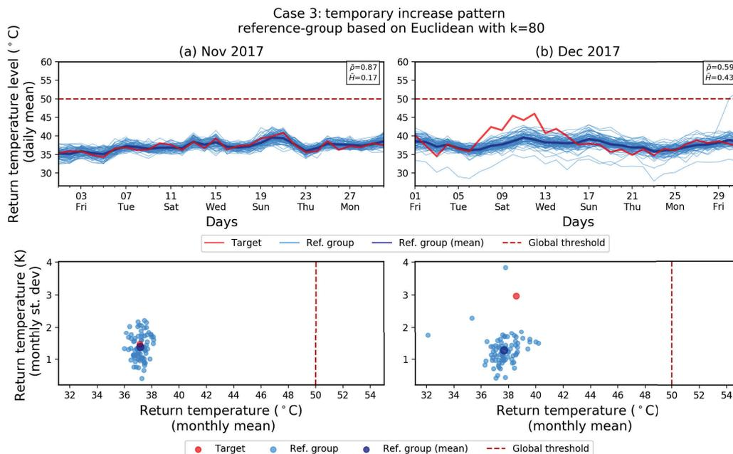
**Figure 8:** Example case of the "temporary increase" pattern: The return temperature of the target shows a considerable increase for about a week compared to its reference-group. A possible reason could be a control malfunction for short duration in Dec'17.
