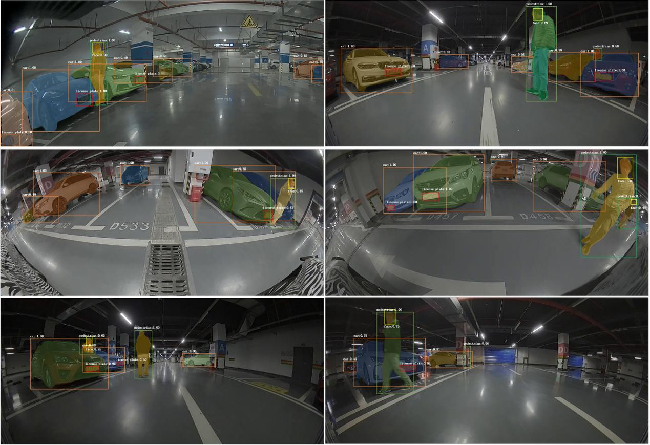
**Figure 8:** Visualized results of our desensitization method on ADD's mixD test set. Green represents the pedestrian detection frame, orange represents the car detection frame, red represents the license plate detection frame, and yellow represents face detection frame. Other masks, such as pedestrian, car, face, and vehicle license plate, are masks after segmentation.
