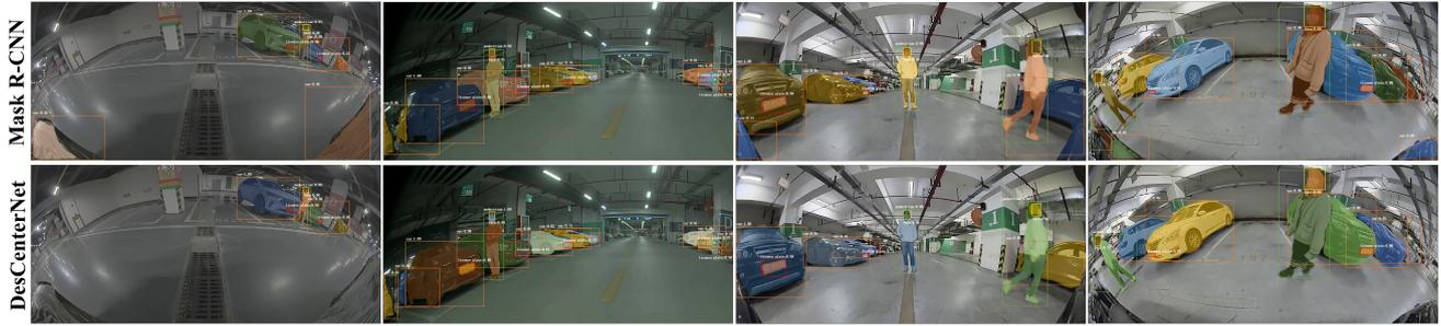
**Figure 4:** Mask R-CNN (top) vs. DesCenterNet (bottom, Hourglass-104). Mask R-CNN has a false detection problem at the edge of the image.
