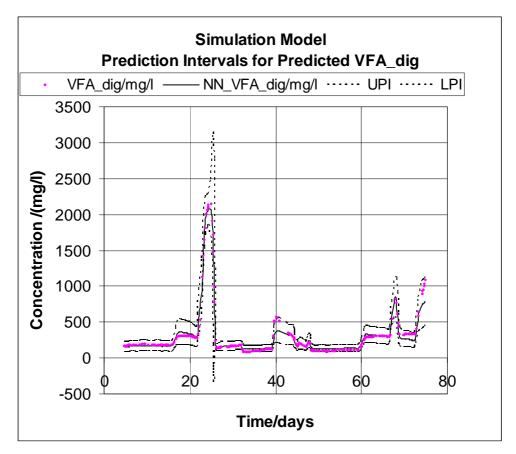
Figure 3: Results of applying neural net model of VFA\_dig
