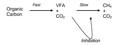
Figure 1: The anaerobic digestion process
