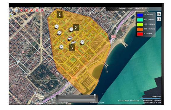
Figure 6 Example of the GIS viewer displaying the following layers : street layer, DMA network wrapping area (label '1'), DMA network pipes coloured according to their diameter, DMA network sensors distinguishing between the inner pressure sensors (label '2') and the pressure / flow sensors of the DMA inlets (label '3').
