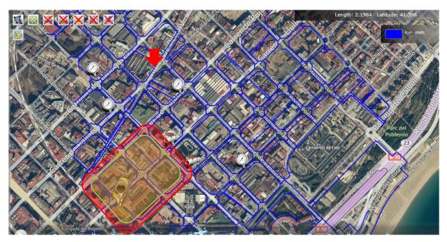
Figure 9 DSS GIS viewer: leakage localization analysis after the 6 l/s leakage was found (*red arrow*) highlighting in a green square area the most rated localizations proposed by the DSS and in red square area the known localizations of the remaining leaks (4 l/s).
