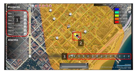
Figure 7 Visualization of the analysis results obtained for a given run: list of available runs (label '1'), resulting most likely leak locations for a given time instant (label '2'), shift bar to visualize the results obtained in every time instant of the selected run (label '3').
