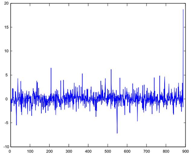
Fig. 13. Damage index variation of unknown damage 1.
