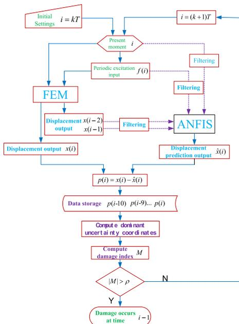
Fig. 12. Flow chart of structural damage identification.
