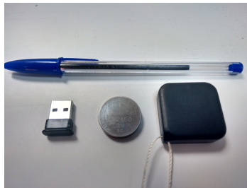
Fig. 1. The BLE advertiser (right), receiver (left), and a power cell CR2450, that is inside the advertiser (center). The pen is shown to compare the sizes.
