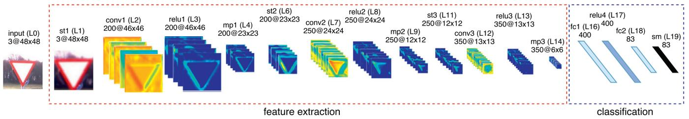
**Fig. 7.** DNN for traffic sign recognition proposed. Local contrast normalization layers have been omitted in the figure above to simplify its visualization as well as localization networks of spatial transformers. The *st* layers refer to spatial transformer networks, *conv* to convolutional layers, *mp* to max-pooling layers, *fc* to fully-connected layers and *sm* to soft-max layer.
