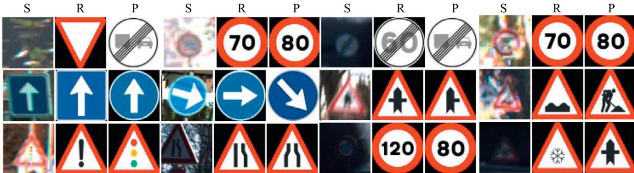
**Fig. 9.** Misclassified samples. Some misclassified samples of the Mixset model trained. As may be seen, the main reason behind them are occlusions and blurred pictographs, being their recognition even hard for the human visual system. Columns labeled with *S* refer to sample, *R* to real traffic sign category and *P* to prediction.
