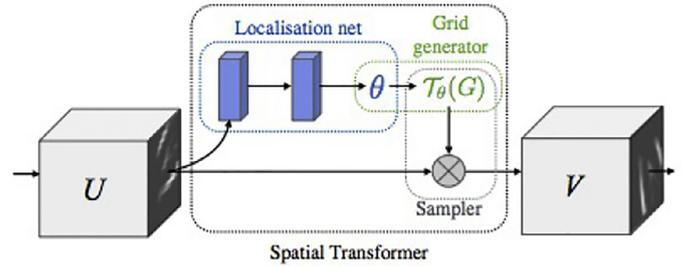
Fig. 6. Spatial transformer network components (Jaderberg et al., 2015).
