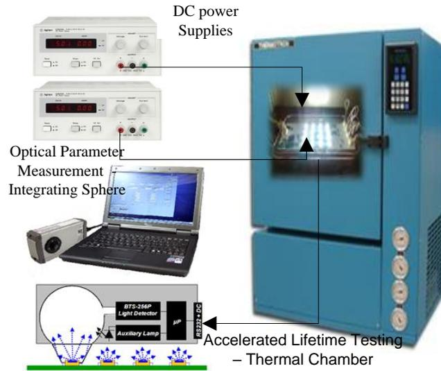
Figure 4. Accelerated Testing Experimental Setup for data collection
