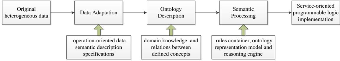
Figure 6: Implementation process of data semantic fusion model.
