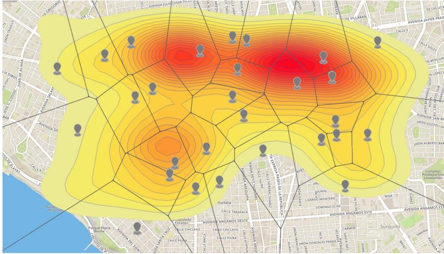
Figure 6: Heatmap of energy transformer substations in Lima compared to the solution of the case study.
