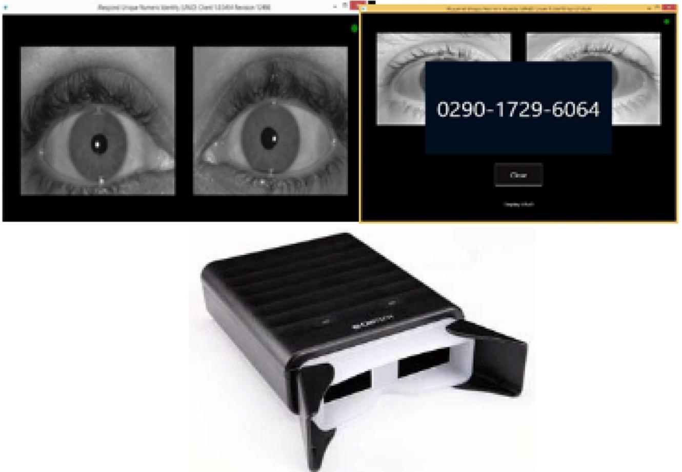
**Fig. 1.** Iris Scan, Camera and ID generation as it appears on screen.
