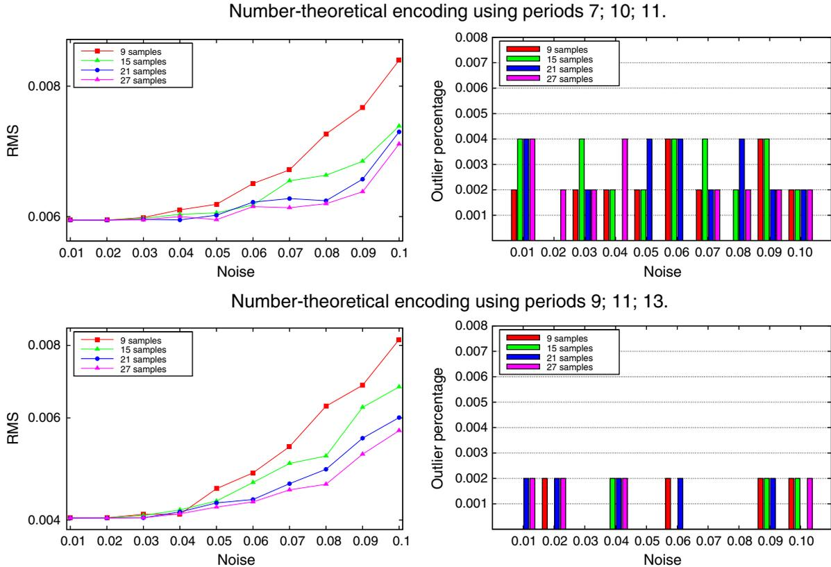
Fig. 5. Precision and robustness to noise of the number-theoretical encoding strategy in conjunction with the subpattern generation strategy. Left: code RMS as a function of the standard deviation of the noise. Right: percentage of outliers (codes with error greater than 1 projector pixel) as a function of the standard deviation of the noise. Same color represents same coding scheme.
