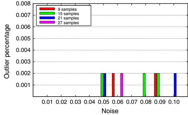
Algebraic encoding using quantizations 8; 10; 10 and evenly distributed samples.
