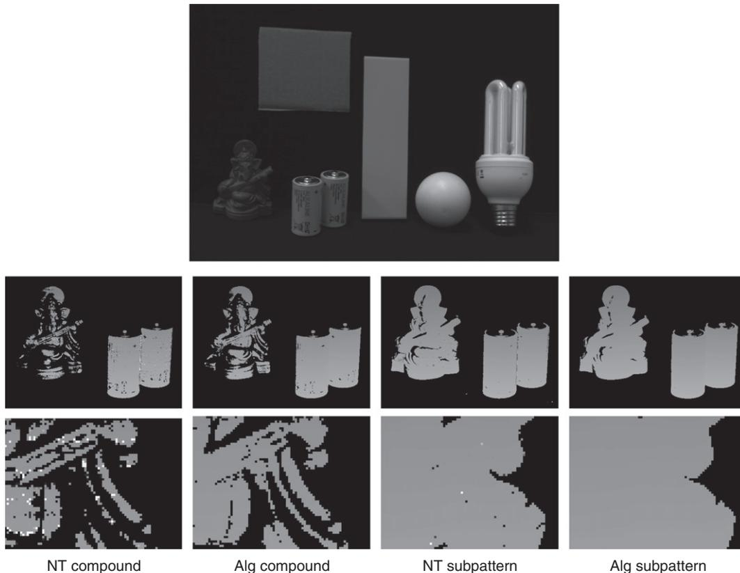
**Fig. 8.** Test scene and example code images with respective close-ups for the number-theoretical and algebraic coding. Grey levels represent the detected code, from 0 (black) to 800 (white). Uncoded pixels are black.
