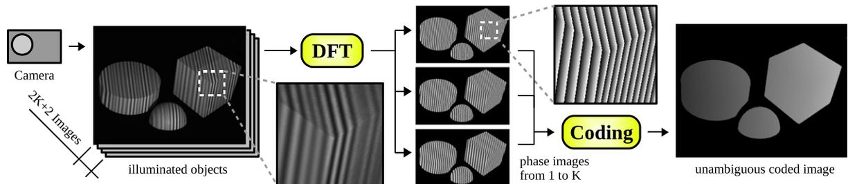
**Fig. 3.** A total of  $2k + 2$  images of illuminated objects are captured and single phase values are calculated for each composed fringe signal. Those values are subsequently used to get an unambiguous coding. Note that the intensity profile of each projected pattern is not sinusoidal.
