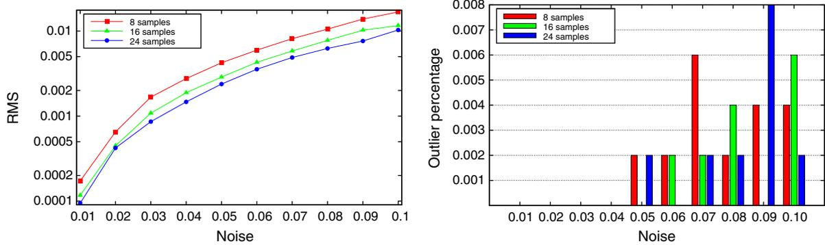
Fig. 7. Precision and robustness to noise of the encoding strategies under study in conjunction with the compound pattern generation strategy. Left: code RMS as a function of the standard deviation of the noise. Right: percentage of outliers (codes with error greater than 1 projector pixel) as a function of the standard deviation of the noise. Same color represents same coding scheme.
