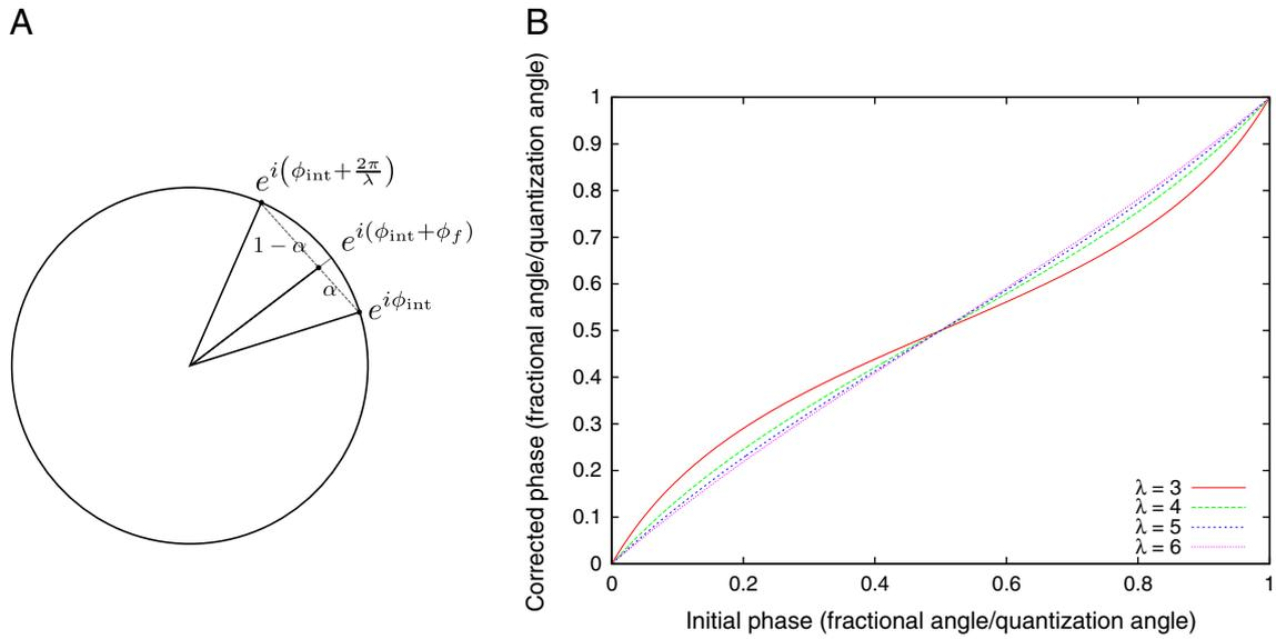
**Fig. 4.** The linear interpolation of the phase/amplitude vectors at adjacent quantized angles does not result in a linear interpolation of the angles. This requires a correction for the fractional part of the phase.
