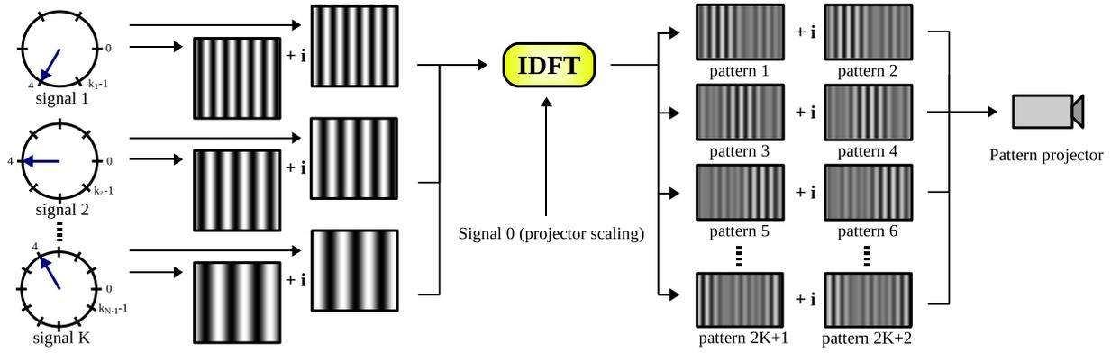
**Fig. 2.** The composition of  $k$  fringe patterns, plus one unknown shift signal will produce a total of  $2(k + 1)$  image patterns that will be projected onto the surface to be reconstructed. The shift pattern (projector scaling) accounts for the unknown value of the albedo of the surface.
