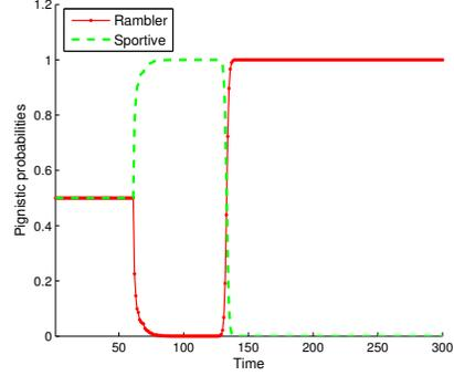
Figure 23: Instantaneous belief ( $m_k$ ) discounting, with  $\lambda = 0.9$ .
