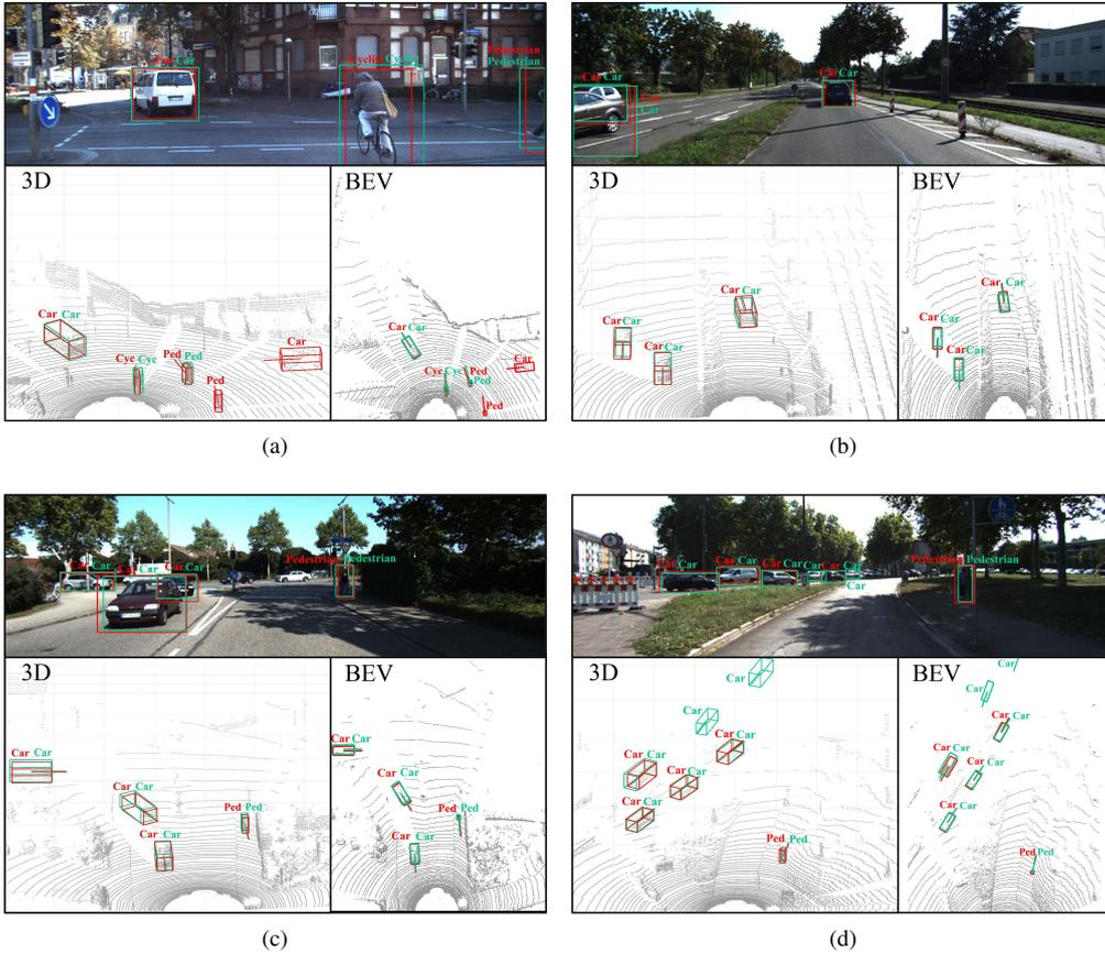
Figure 9: **The results of our algorithm.** The red boxes represent our detection results, and the green boxes represent the groundtruth. In each subgraph, the bottom-left part shows 3D results, and the bottom-right shows the BEV results.
