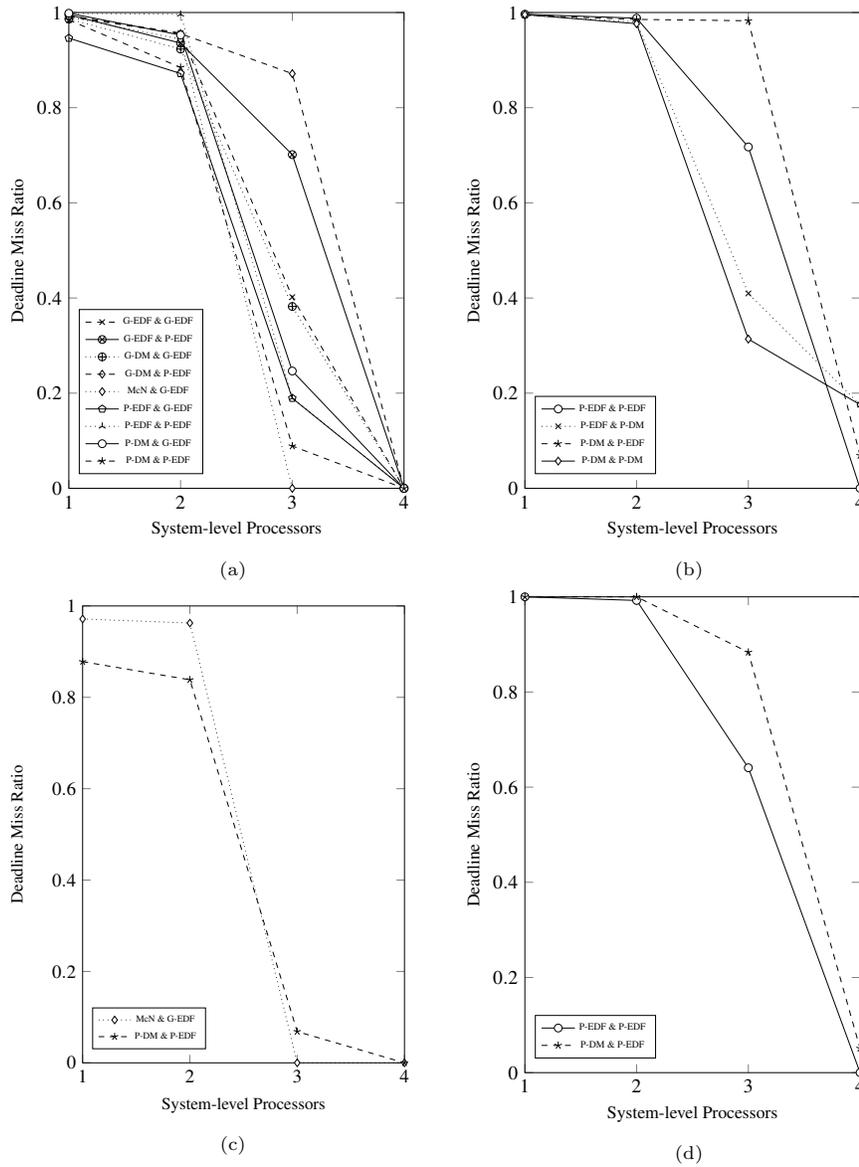
Figure 4: In Figures a & b the results are displayed from the simulation-based analysis for respectively application 1 & 2. Figures c & d display the results of the analysis with Xvisor-RT for the selected scheduling algorithms.
