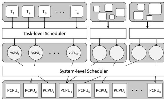
Figure 1: Visual representation of a hierarchical scheduling structure on a multi-core platform.
