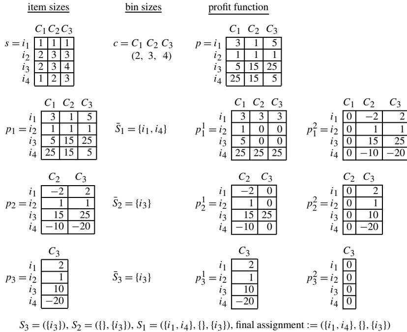
Fig. 1. Algorithm 1—running example for 4 items.
