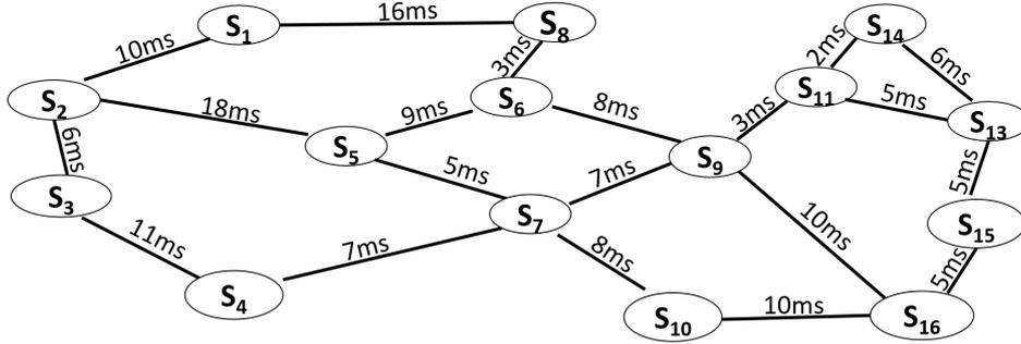
Figure 5: Example network composed of sites  $\{S_1, \dots, S_{16}\}$ . Edges correspond to communication links among them, while network latency values (in milliseconds) are noted on the links.
