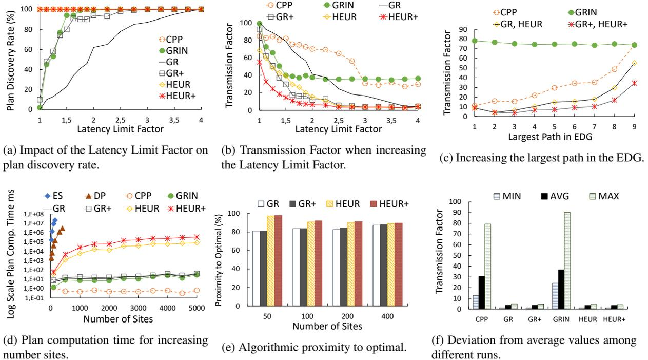
Figure 10: Cost, Time and quality sensitivity analysis on various network, EDG and optimization related parameters.
