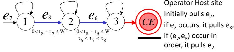
Figure 3: A three-step NFA for the  $\text{SEQ}(e_6, e_7, e_8)$  operator of Figure 1.  $W$  denotes the time window of the operator, while  $t_i$  denotes the timestamp of event  $e_i$ . Constraints on NFA edges are present in order to ensure correctness.
