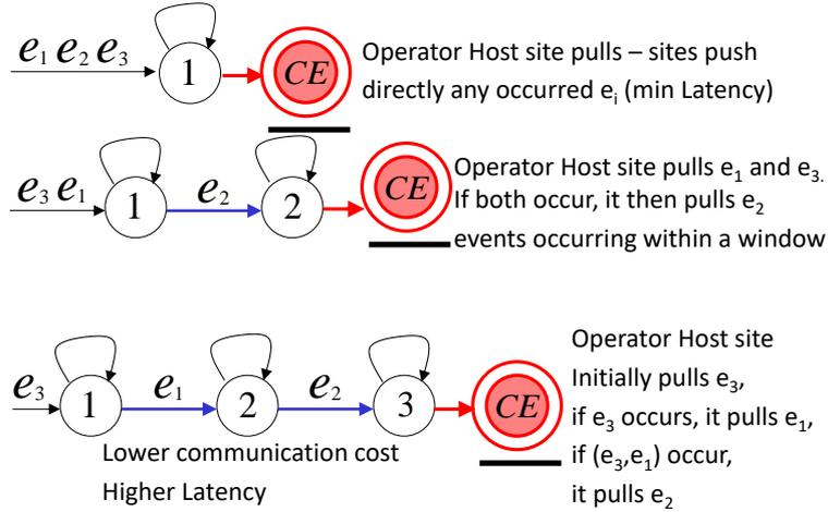
Figure 2: Three alternative NFAs for different push-pull orderings for the AND operator of Figure 1. Self-transiting edges are used for the occurrence of  $e_i$ 's at the corresponding state. Blue edges represent events that may be pulled. Pulling events reduces bandwidth, but increases latency.
