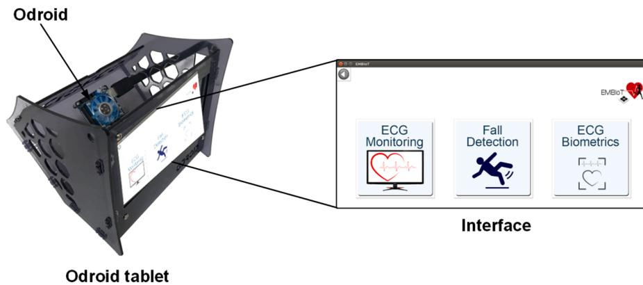
Fig. 10. System runs on ODROID IoT device with touch screen.
