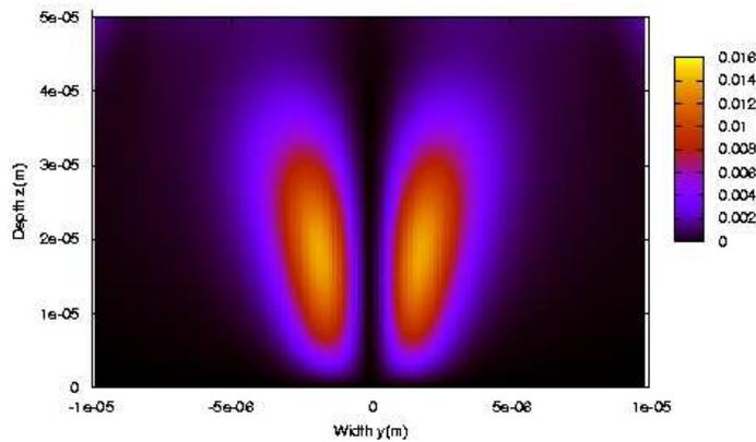
Figure 16. Energy flux  $F_x$  in a SHG experiment without phase matching after a propagation in  $50\mu\text{m}$  of KDP (268 fs). We have used the same arbitrary units for the intensity as in Fig. 15.
