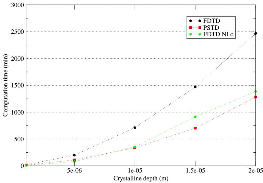
Figure 8. Computation times for the three schemes (PSTD=pseudospectral scheme, NLc=FDTD scheme of Sec. 3.3) for several crystalline lengths on an Intel<sup>®</sup> Xeon<sup>™</sup> 2.2 GHz.
