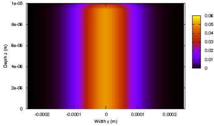
Figure 11. Energy flux  $F_y$  in a SHG experiment at the phase matching angle after a propagation in  $10\mu\text{m}$  of KDP. We have used arbitrary units for the intensity.
