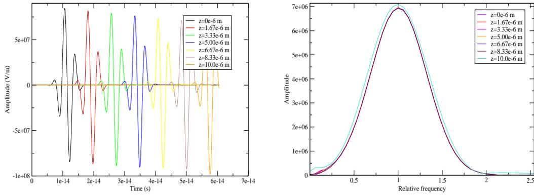
Figure 13. The  $E_y$  component and its Fourier transform in an experiment of second harmonic generation for seven points in the crystal. The amplitude of the Fourier transform is plotted in arbitrary units, the frequency is relative to the one of the incoming beam.
