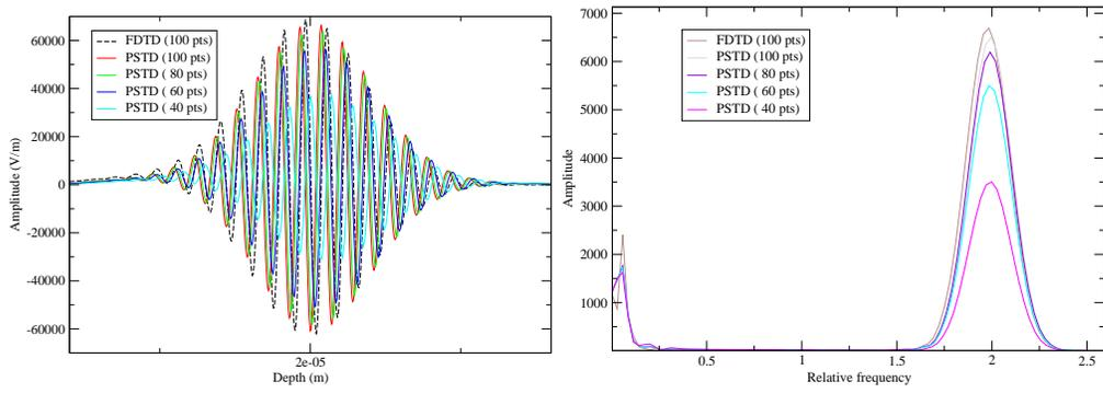
Figure 9.  $E_x$  component and its Fourier transform in an experiment of second harmonic generation using the pseudospectral (PSTD) scheme for several sizes of the space step. For comparison, we have also plotted the result obtained by the scheme of Sec. 3.1 (FDTD). The frequency is relative to the frequency of the incoming wave-field.
