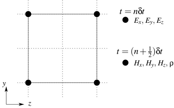
Figure 3. Pseudospectral scheme for the electromagnetic wave ( $\mathbf{E}, \mathbf{H}$ ) and the density matrix  $\rho$ .
