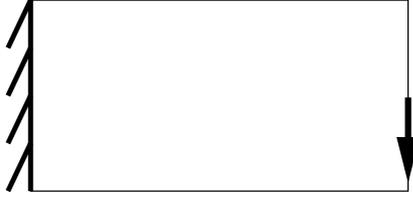
Figure 2. Boundary conditions for the cantilever.
