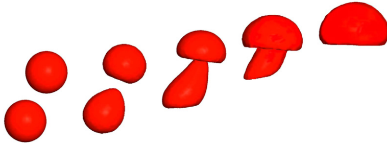
Fig. 18. Transient solution of bubble coalescence when the bubbles are not aligned. Fr = 1 , Re = 18.8 , We = 50 , \rho_1/\rho_2 = 26 , \mu_1/\mu_2 = 20 . From left to right the non-dimensional time is t^* = 0 , t = 0.5 , t = 1 , t = 1.5 , t = 2 .
