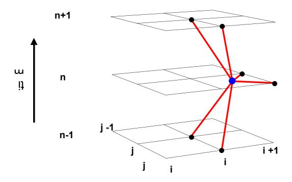
Fig.1: Grid points involved in the computation of the heat fluxes at point (i+1/2,j+1/2) required for the DuFort-Frankel scheme used along the sub-domain boundary at  $r=r_i$  (along the "DuFort-Frankel line").
