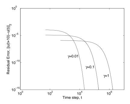
Fig. 2. Convergence histories (in log-log scale) of preconditioned MRT-LBE with forcing term for simulation of Poiseuille flow with maximum flow velocity  $u_{max}=0.0128$  and kinematic viscosity  $\nu=0.005;\ Re=163.8.$
