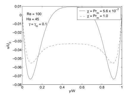
Fig. 19. Effect of magnetic Prandtl number  $Pr_m$  on computed velocity profile u along the line x = W/2 and z = W/2 for simulation of 3D cubical lid-driven cavity in the presence of magnetic field perpendicular to the lid surface and its direction of motion; Re = 100 and Ha = 45.
