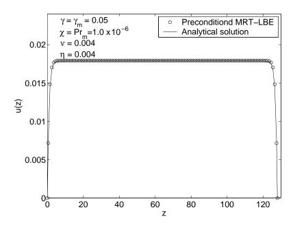
Fig. 6. Comparison of computed velocity profile using the preconditioned MRT-LBE with analytical solution for simulation of Hartmann flow with preconditioning parameters  $\gamma = \gamma_m = 0.05$  and kinematic viscosity  $\nu = 0.004$ ; Re = 286, Ha = 71.6.
