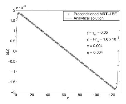
Fig. 7. Comparison of computed induced magnetic field profile using the preconditioned MRT-LBE with analytical solution for simulation of Hartmann flow with preconditioning parameters  $\gamma = \gamma_m = 0.05$  and kinematic viscosity  $\nu = 0.004$ ; Re = 286, Ha = 71.6.
