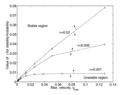
Fig. 5. Parameter space of the preconditioning parameter  $\gamma$  for stable/unstable computations using the preconditioned MRT-LBE for simulation of Poiseuille flow at different maximum possible flow velocities  $u_{max}$  and kinematic viscosities  $\nu$  of the fluid.
