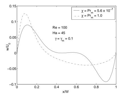
Fig. 20. Effect of magnetic Prandtl number  $Pr_m$  on computed velocity profile u along the line y = W/2 and z = W/2 for simulation of 3D cubical lid-driven cavity in the presence of magnetic field perpendicular to the lid surface and its direction of motion; Re = 100 and Ha = 45.
