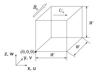
Fig. 11. Schematic illustration of a three-dimensional (3D) cubical cavity with its top lid moving at velocity  $U_0$  in the presence of an external magnetic field  $B_0$ , applied parallel to the lid surface and perpendicular to its direction of motion.
