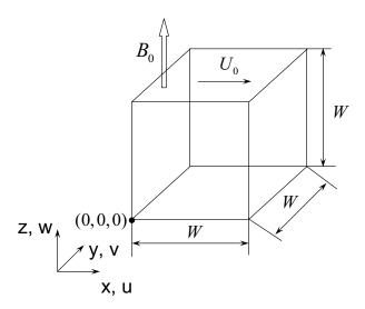
Fig. 17. Schematic illustration of a three-dimensional (3D) cubical cavity with its top lid moving at velocity  $U_0$  in the presence of an external magnetic field  $B_0$ , applied perpendicular to both the lid surface and its direction of motion.
