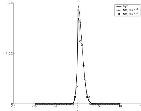
Figure 8: **Test case 3.** Velocity histogram with respect to the first component of the microscopic velocity in  $x = 0.5$  at  $t = 0.12$  for the NB3 scheme (circles), NB4 scheme (dotted line), and for the hybrid algorithm (continuous line)
