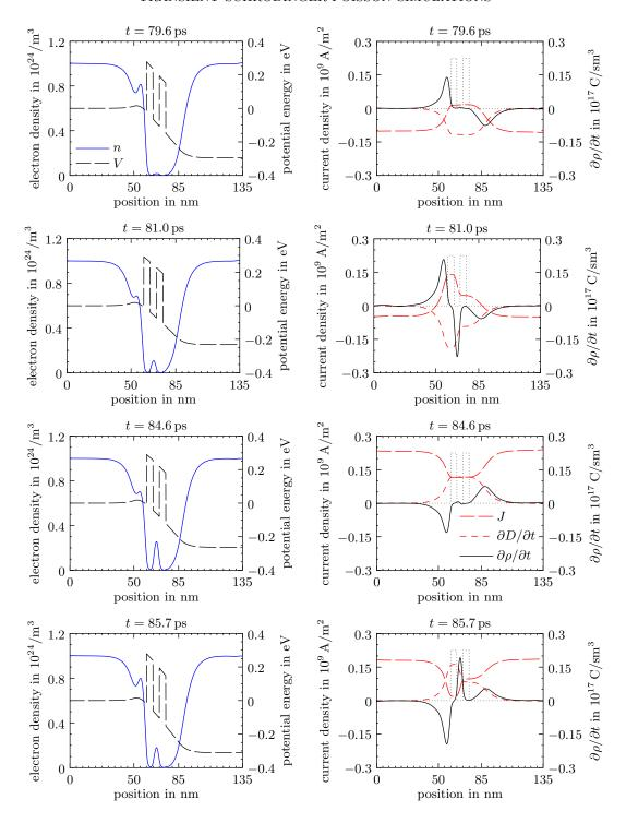
FIGURE 14. First circuit simulation: Electron density, potential energy, current densities, and variation of the electron density versus position in the RTD at four different times.
