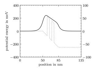
FIGURE 2. Left part: Solid line: self-consistent solution  $V_{\text{self}}$  for  $U = 0 \,\text{mV}$ , found after 7 iterations. Dashed lines: divergent approximations for  $U = 1 \,\text{mV}$ . Dotted line: barrier potential. Right part: Solid line: self-consistent solution  $V_1$  for  $U = 250 \,\text{mV}$  according to approximation (10). Dotted line: sum of the barrier potential and a ramp-like potential.
