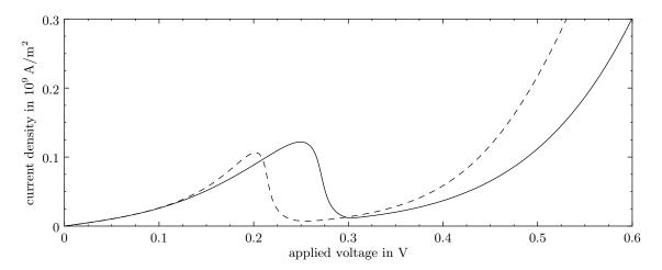
FIGURE 4. Current-voltage characteristics. The solid line corresponds to our solution of the original stationary Schrödinger-Poisson system. The dashed line is obtained with the modified model using approximation (10).
