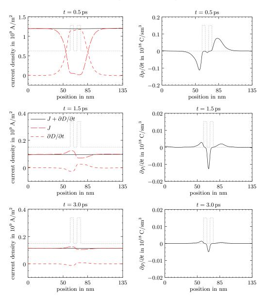
FIGURE 7. Left column: Total current density  $J_{\rm tot} = J_{\rm cond} + \partial D/\partial t$ , conduction current density  $J := J_{\rm cond}$ , and displacement current density  $\partial D/\partial t$  versus position at different times. Right column: Temporal variation  $\partial \rho/\partial t$  of the charge density versus position.
