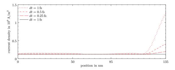
FIGURE 6. Conduction current density in a resonant tunneling diode at  $t=25\,\mathrm{fs}$  for a constant applied voltage of  $U=250\,\mathrm{mV}$ . Discretizations using the ad-hoc discretization (19) of the analytical boundary conditions yield strongly distorted numerical solutions (broken lines). In contrast, the conduction current density computed with our solver is perfectly constant (solid line).
