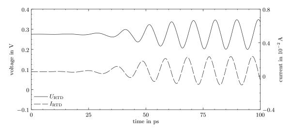
FIGURE 15. Second circuit simulation: Applied voltage and current at the resonant tunneling diode versus time.
