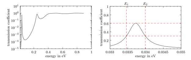
FIGURE 10. Transmission coefficient of the double-barrier structure at  $U = 0.25 \,\mathrm{V}$  in different scalings.
