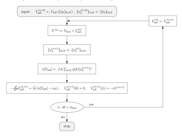
FIGURE 5. Flow chart of the transient scheme.
