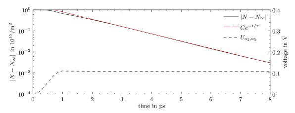
FIGURE 9. Number of electrons in the quantum well versus time. In Region III  $(t \ge 2 \text{ ps})$  this number clearly follows an exponential law.  $U_{a_2,a_5}$  denotes the temporal variation of the voltage between  $x = a_2$  and  $x = a_5$ .
