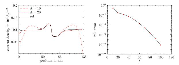
FIGURE 11. Conduction current density at  $t = 1.5 \,\mathrm{ps}$  (left) and relative  $\ell^2$ -error for increasing  $\Lambda$ .
