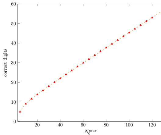
Figure 3: Correct digits of the lowest eigenvalue of the L-shaped membrane obtained with Richardson extrapolation using a set of FD grids with a smallest spacing  $h_{min} = 1/N_0^{max}$ . Notice that the number of grids used for a given  $h_{min}$  depends on  $h_{min}$  itself (see Fig. 4). The dashed curve is the fit  $f(n) = 7.23166 + 0.383229n - \frac{20.9176}{n}$ . The FD eigenvalues used in the extrapolation were computing using 220 decimal digit floating point arithmetic.
