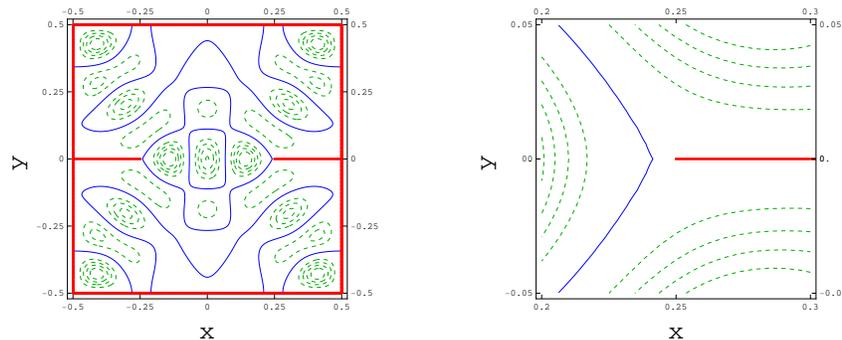
Figure 14: Nodal lines of the 50<sup>th</sup> mode of the square domain with two slits.
