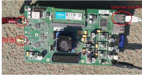
Figure 14: The WARP system photo.
