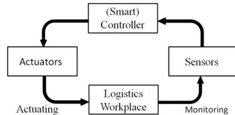
Fig. 1. A Smart Closed-loop System for Workplace Safety
