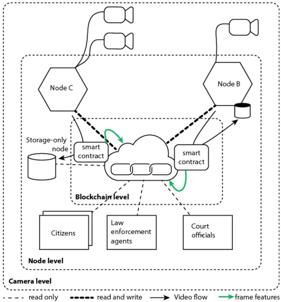
**Figure 6:** Blockchain-enabled Video Surveillance in a Smart City
