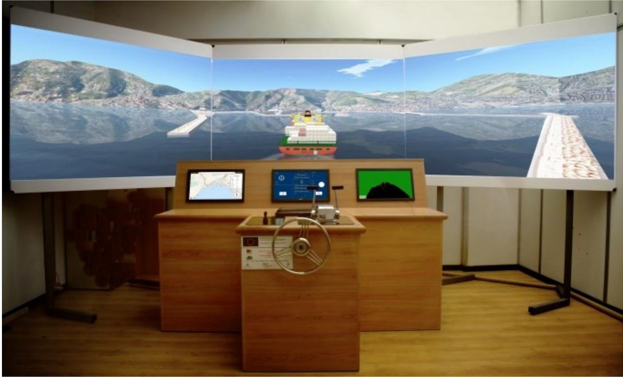
Figure 21: The ship bridge replica and the visualization area
