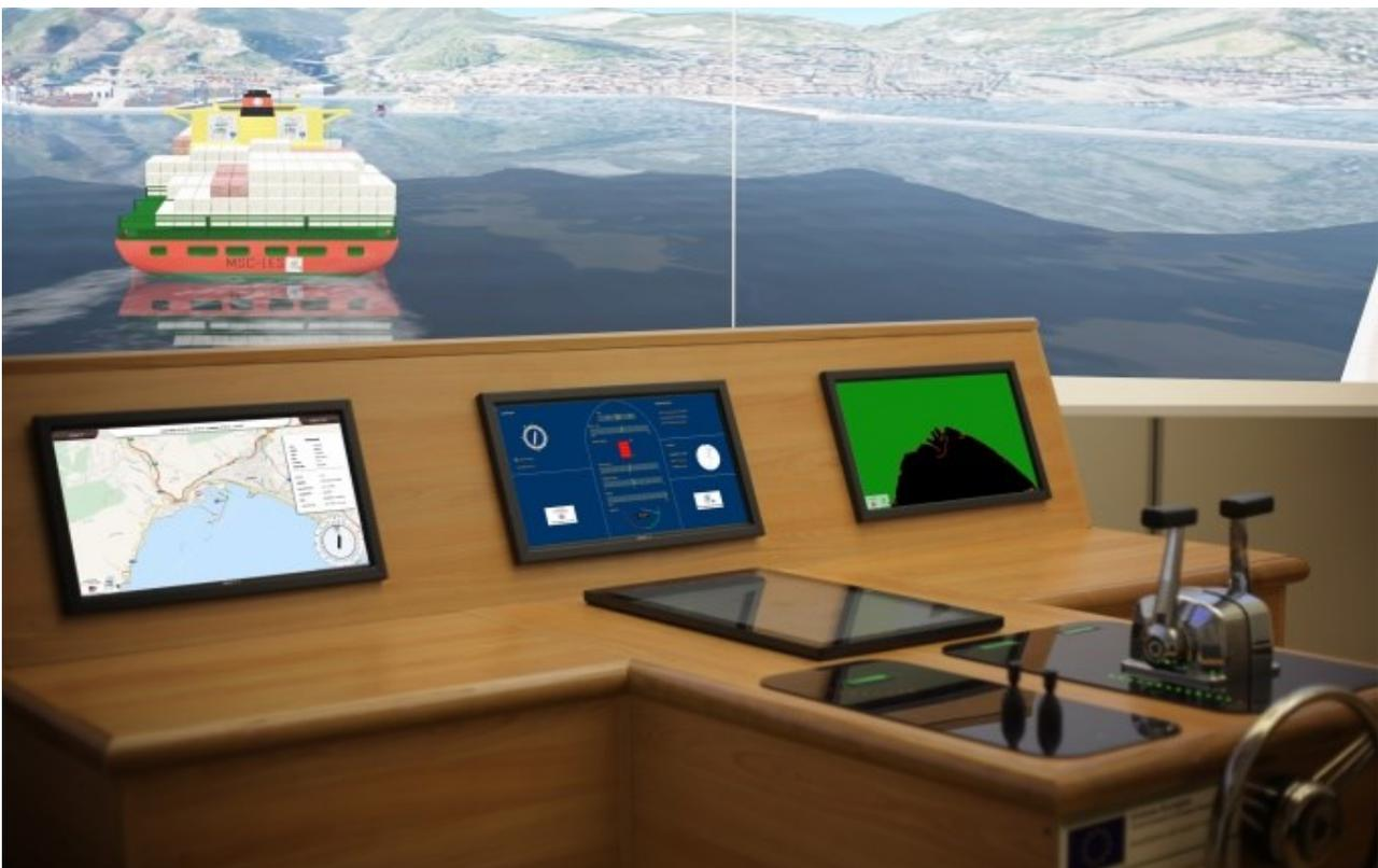
Figure 16: Ship bridge detail: navigation instruments and visualization area including AIS simulator, Conning display simulator, Radar simulator
