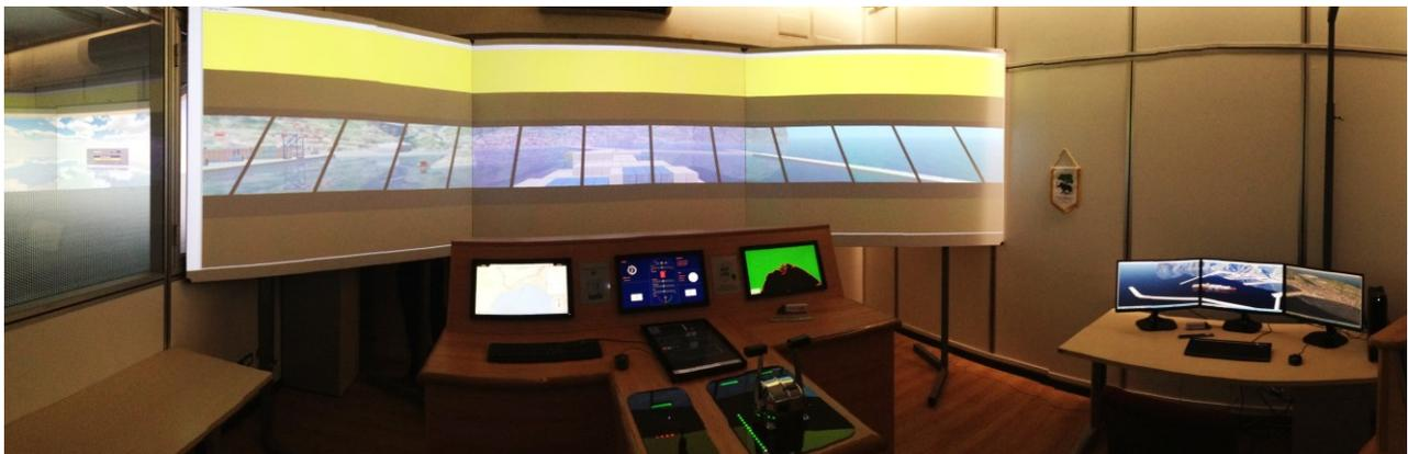
Figure 22 – The ship bridge simulator and the control tower simulator working together for cooperative training of ship pilots and port traffic controller (Interoperability use mode and distributed simulation through High Level Architecture)
