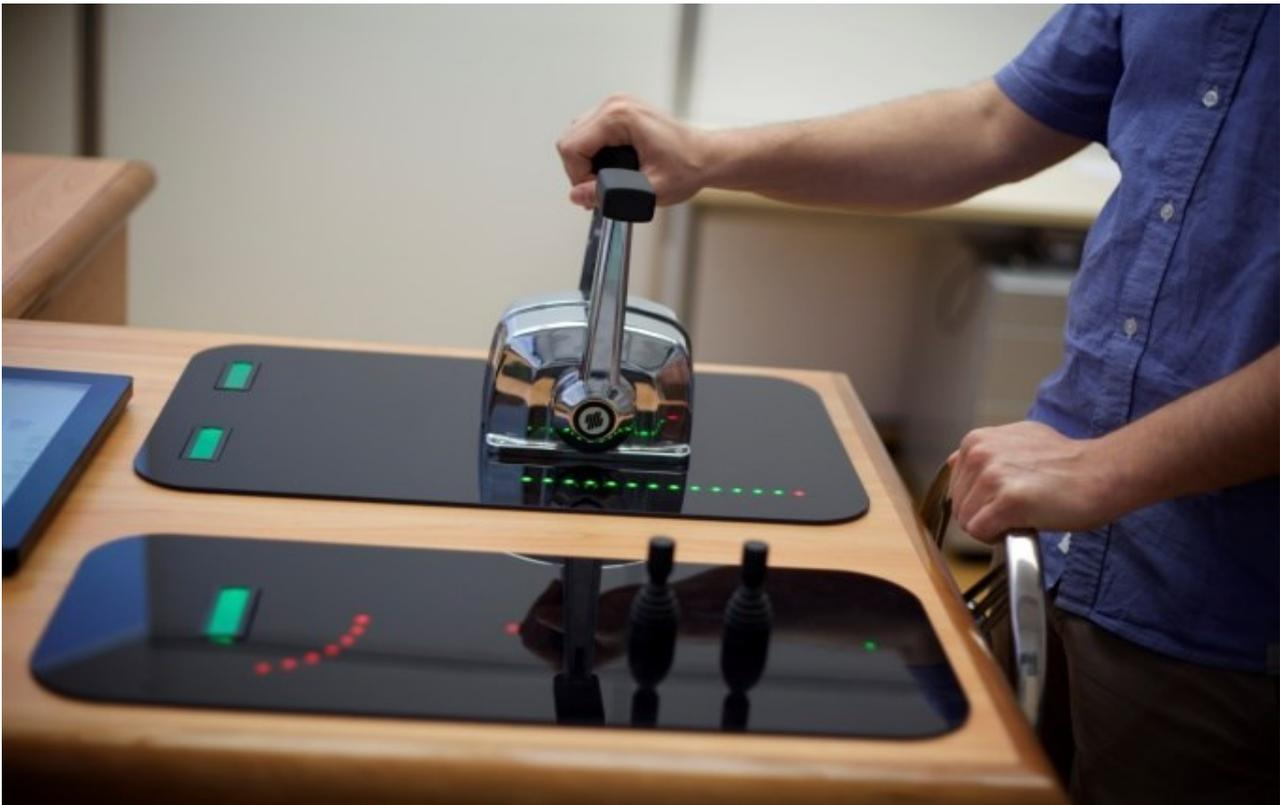
Figure 15: Ship bridge detail: double lever system, joysticks for side thruster control, wheels for rudder control, multiple LEDs displays and small-size displays
