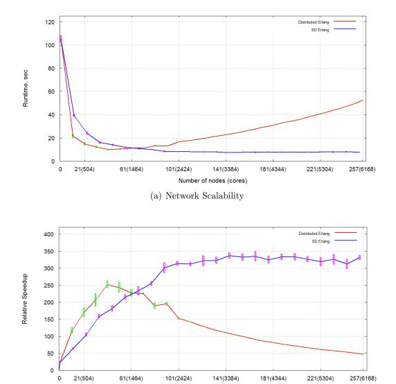
Figure 9: Impact of Transitive Connections on Network Scalability of Distributed and SD Erlang Orbit
