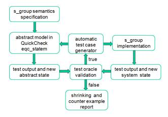
Figure 6: Testing s\_groups Using QuickCheck
