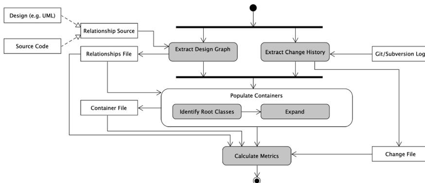
Figure 7 Automated Container Analysis Tools
