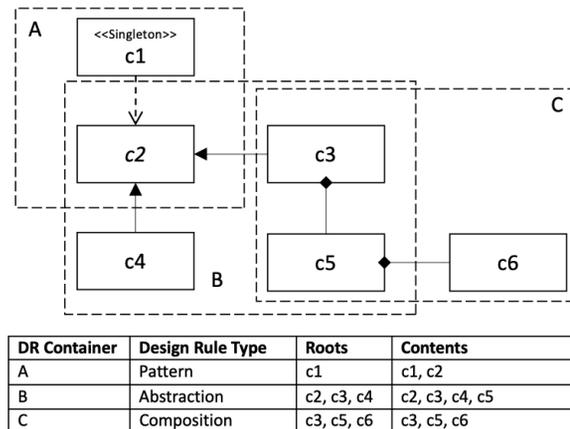
Figure 1 Design Rule Container Example
