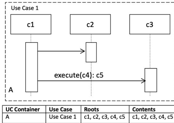
Figure 3 Use Case Container Example
