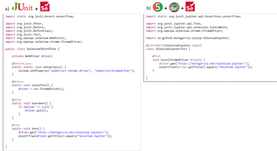
Figure 5: Comparison of Selenium WebDriver tests using local web browsers with: a) JUnit 4. b) JUnit 5 and Selenium-Jupiter
