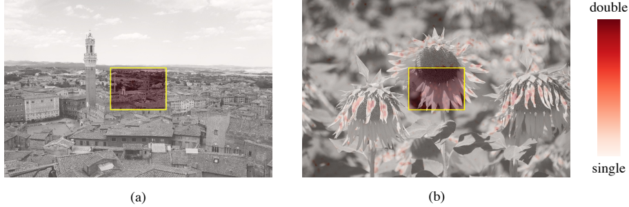
Figure 10: A-DJPEG (a) and NA-DJPEG (b) localization example of a compressed central region with QF2 = 95 and QF1 = 80 . \mathcal{C}_{\text{hist}} is used for the aligned case while \mathcal{C}_{\text{noise}} for the non aligned case. Actual forged region lies inside the yellow rectangle.
