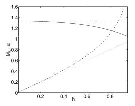
Figure 2. The graph shows the dependence of the kink mass  $M_k$  given by Eq. (24) (solid line) as a function of the lattice spacing h. The continuum limit corresponding to  $M_k = 4/3$  (see the main text) is shown by the dash-dotted line. The dashed line illustrates the dependence of the parameter  $\alpha$  on the spacing h, while the dotted line shows the linear behavior for comparison.
