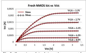
Fig. 3. Comparison of simulation and measurement for fresh NMOS, I<sub>DS</sub> vs. V<sub>DS</sub>
