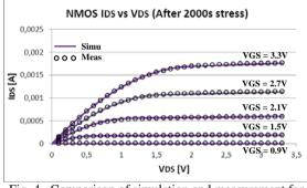
Fig. 4. Comparison of simulation and measurement for NMOS after 2000s HCI stress, I<sub>DS</sub> vs. V<sub>DS</sub>
