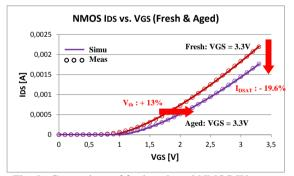
Fig. 5. Comparison of fresh and aged NMOS IV curve  $(I_{DS} vs. V_{GS})$  for measurement and simulation
