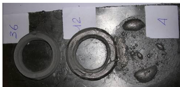
Fig. 11. Toroid samples after the sintering process.
