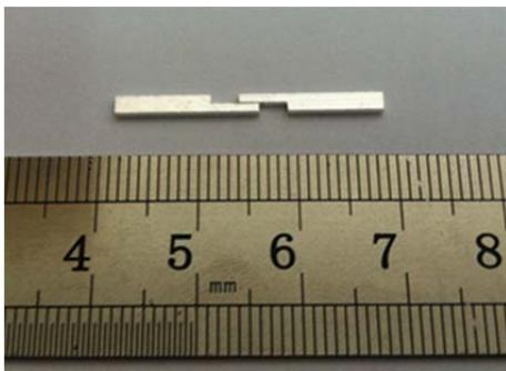
Fig. 1 Prepared sintered nano-silver lap-shear structure
