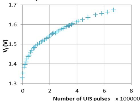
Fig. 11. Evolution of body diode forward voltage (V<sub>f</sub>) as a result of repetitive UIS stress
