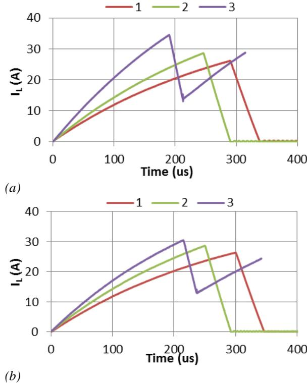
Fig. 4. Single pulse UIS waveforms at  $T_{CASE}$  (a)  $90^{\circ}C$  and (b)  $150^{\circ}C$ ,  $V_{DD} = 400V$  with various  $L$  values and constant  $E_{AV}$
