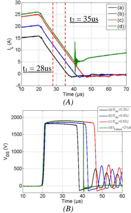
Fig. 8. UIS electrical waveforms: (A)  $I_L$  and (B)  $V_{DS}$ , with  $T_{CASE} = 27^{\circ}C$ ;  $L = 1.8mH$ ; (a)  $V_{DD}=140V$ ,  $t_{ON} = 200\mu s$  (b)  $V_{DD}=180V$ ,  $t_{ON}=200\mu s$  (c)  $V_{DD}=200V$ ,  $t_{ON}=220\mu s$ ; (d)  $V_{DD}=200V$ ,  $t_{ON}=230\mu s$ .
