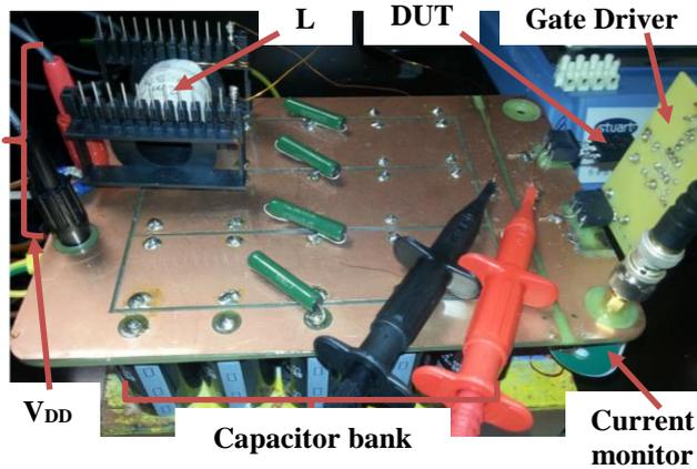
Fig. 2. UIS test circuit
