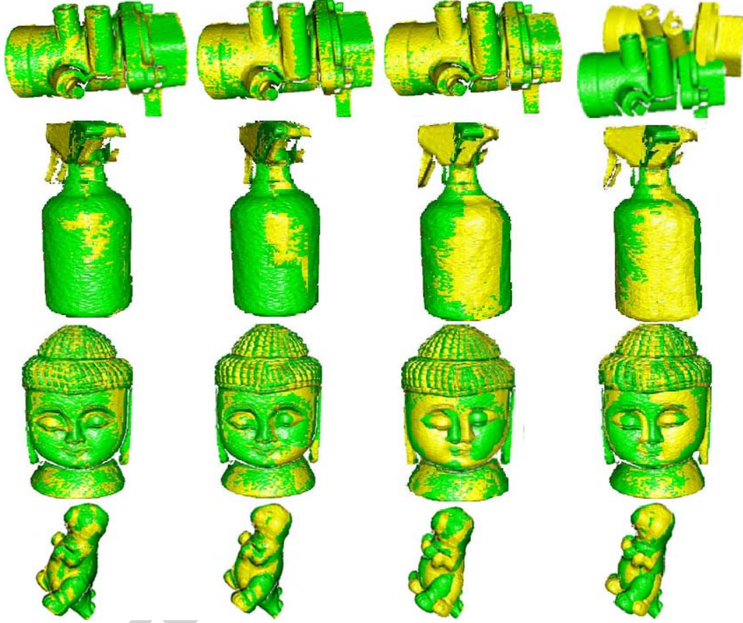
Figure 10: Registration results using the FICP algorithm of the interest points detected from different scans using different algorithms. Columns, left to right: RBS, OVBS, 3D-SIFT, and 3D-Harris. Rows, top to bottom: valve0-10, bottle144-180, buddha0-20, and dinosaur36-72.
