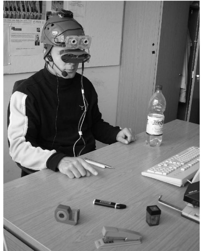
Fig. 1. User with head mounted cameras and display. The input is looped back into the display and enhanced by visual augmentations.
