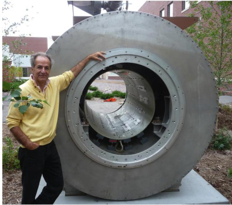
**Figure 2.** The picture shows the author next to the 125 cm bore 4 Tesla magnet from Siemens that was originally installed in CMRR in 1990. This magnet is now a garden “statue” in the courtyard of CMRR, University of Minnesota.
