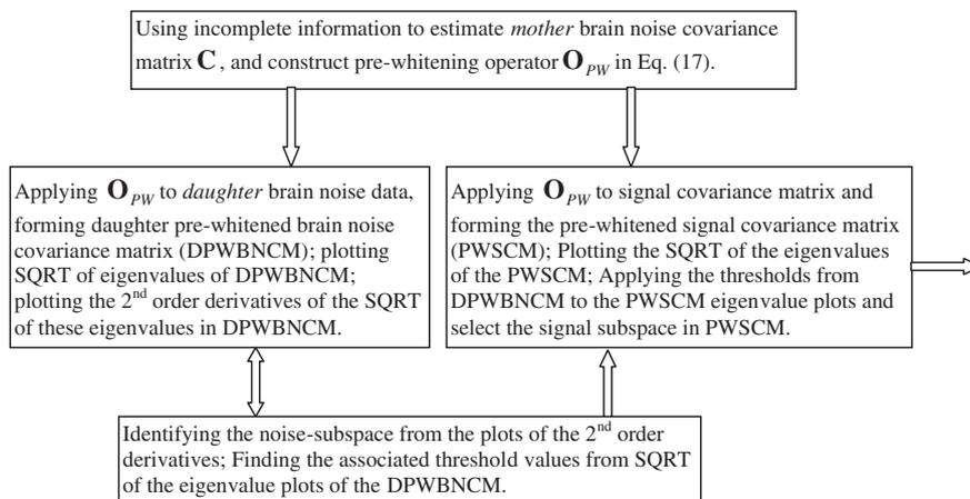
**Fig. 2.** A flow-chart of the objective pre-whitening method (OPWM) for removing correlated brain noise from the data. The same process was applied to remove correlated environmental noise when replacing the DPWBNCM in the chart with the daughter pre-whitened empty-room covariance matrix (DPWERC M).
