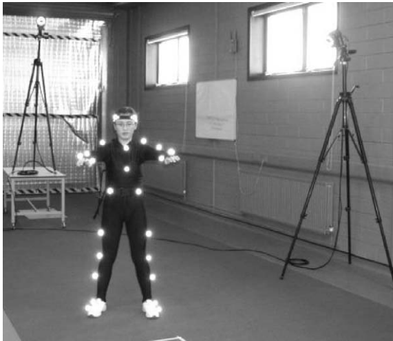
Fig. 1. Capture of 3D human pose data in Vicon-512 system.
