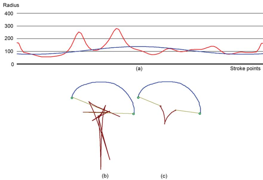
Figure 9. Radius and centers of rotation for the same example in Fig. 8: a) discrete (red) and analytic (blue) radius; b) centers of rotation (brown) for each point of the stroke calculated by means of discrete direction and radius; c) same as b) calculated by means of analytic direction and radius
