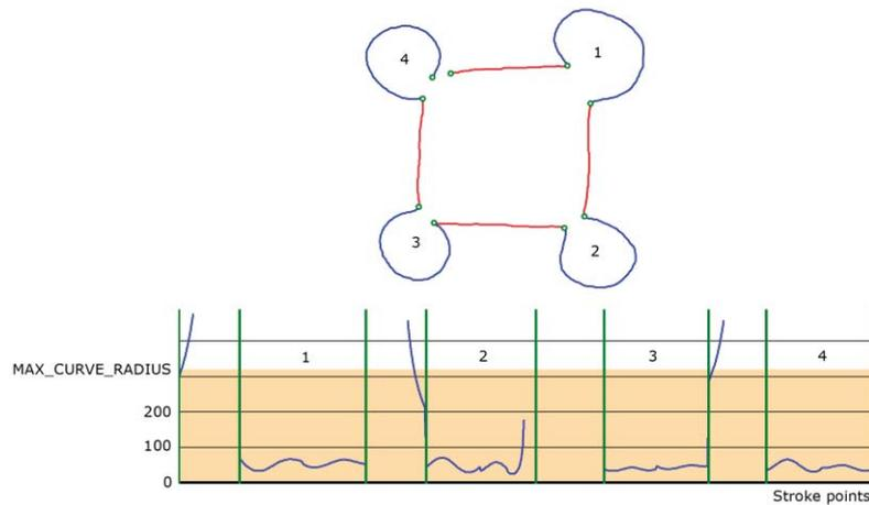
Figure 11. Shape with curves (blue) and straight lines (red) separated by corner vertices.
