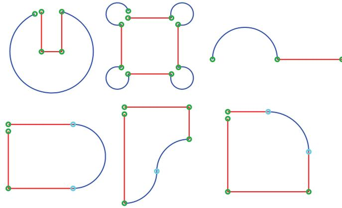
Figure 14. Strokes with straight lines (drawn in red), curves (drawn in blue), corner vertices (drawn in green) and tangent vertices (drawn in blue cyan)
