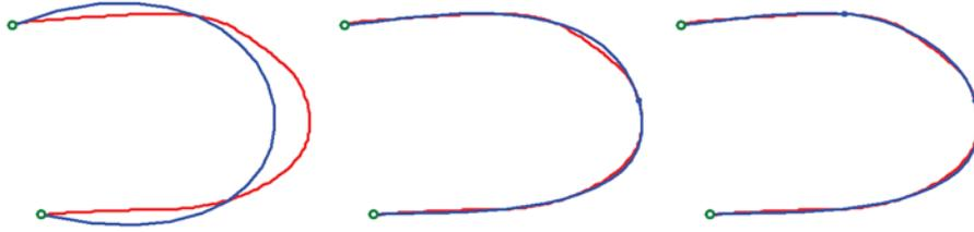
Figure 8. Resampled points of a stroke (red) and piece-wise parametric cubic curves approximation (blue). From left to right, with 1, 2 and 3 parametric cubic curves
