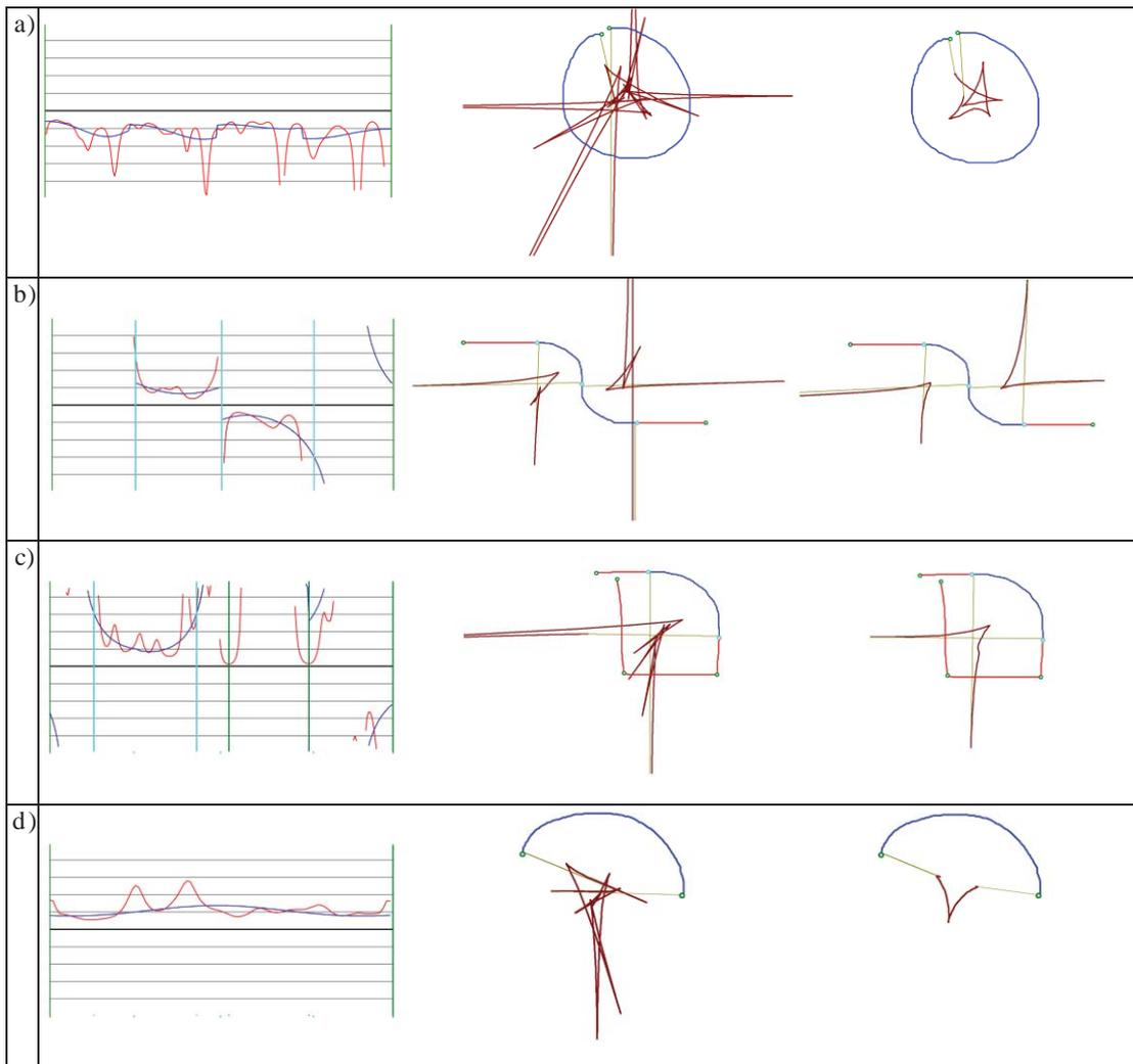
Figure 16. Left column: radius function from original sketched points (red) and from approximated parametric cubic curves (blue); Central column: radius from original sketched points represented (brown); Right column: radius from approximated parametric cubic curves represented (brown), of different samples of sketches a), b), c) and d) respectively
