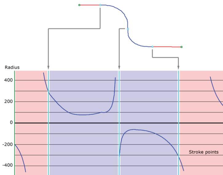
Figure 12. Tangent vertices (drawn in cyan) between curves and straight lines, and between two curves. The background of radius function is blue for curves and red for straight lines
