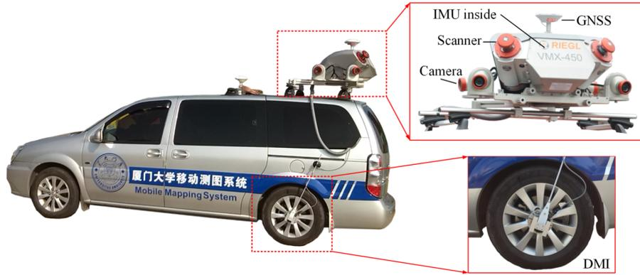
**Fig. 7.** Illustration of RIEGL VMX-450 mobile LiDAR system and its configurations.
